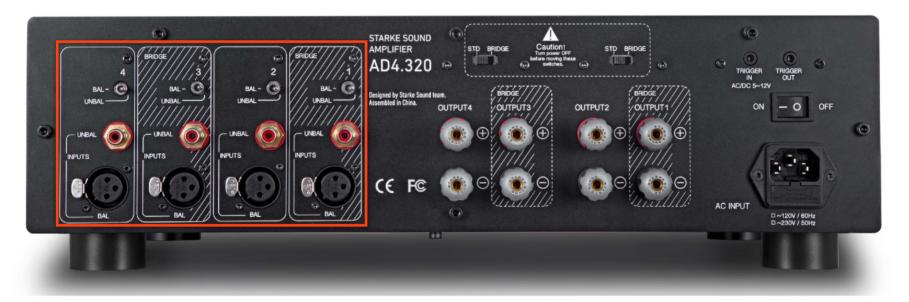
Connect your four speakers to the output binding posts: 1, 2, 3 and 4. Speaker wires can be terminated with "banana plugs" which are inserted, or stripped insulation (unscrew binding post cap, insert wire into hole on threaded shaft and tighten cap). Observe correct polarity ("+" red and "-" black).
