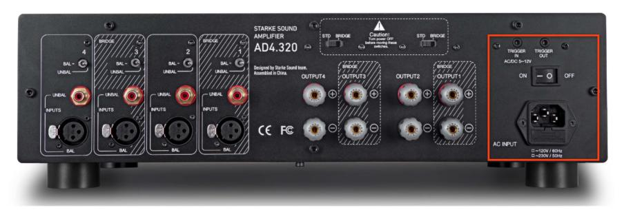
Your AD4.320 can also serve as a 2-channel or 3-channel amplifier, delivering greater power to 2, or to 3 channels. This is done by "bridging." **For 2-channel operation**, first, TURN OFF THE AMPLIFIER. Then, set both switches to BRIDGE.
