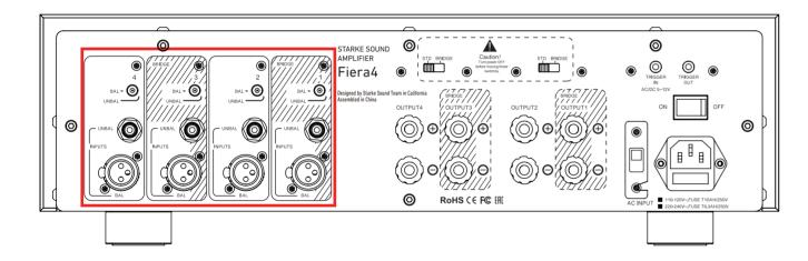
Connect your four speakers to the output binding posts: 1, 2, 3 and 4. Speaker wires can be terminated with "banana plugs" which are inserted, or stripped insulation (unscrew binding post cap, insert wire into hole on threaded shaft and tighten cap). Observe correct polarity ("+" red and "-" black).
