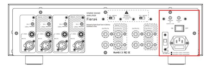
Your Fiera 4 can also serve as a 2-channel or 3-channel amplifier, delivering greater power to 2, or to 3 channels. This is done by "bridging." **For 2-channel operation**, first, TURN OFF THE AMPLIFIER. Then, set both switches to BRIDGE.
