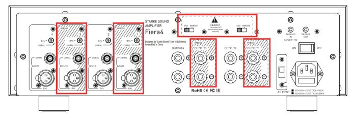
Connect your inputs and outputs to 1 and 3 (INPUTS can be unbalanced RCA or balanced XLR; set toggle switches accordingly and use speaker wire for OUTPUTS). Twice the power will be delivered to OUTPUTS 1 and 3. Only turn on the amp AFTER these changes are made.
