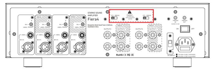
For 4-channel operation, set these two switches to STD (standard).
