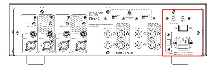
Your Fiera 4 can also serve as a 2-channel or 3-channel amplifier, delivering greater power to 2, or to 3 channels. This is done by "bridging." **For 2-channel operation**, first, TURN OFF THE AMPLIFIER. Then, set both switches to BRIDGE.
