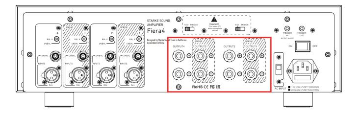
The amplifier can be turned-on automatically by, for example, your preamp/processor by connecting a 12-volt trigger wire to TRIGGER IN. You can use TRIGGER OUT to connect a "downstream" component such as another amplifier to also be turned-on automatically. Connect the power cord to AC INPUT and plug the other end into a 120-volt wall socket. Set the rocker switch to ON to power-on the amplifier.
