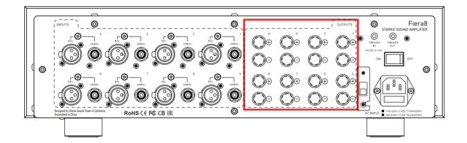
Connect up to 8 speakers to the output binding posts: 1 - 8. Speaker wires can be terminated with "banana plugs" which are inserted, or stripped insulation (unscrew binding post cap, insert wire into hole on threaded shaft and tighten cap). Observe correct polarity ("+" red and "-" black).
