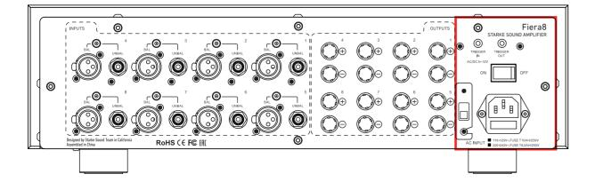
The amplifier can be turned-on automatically by your preamp/processor by connecting a 12-volt trigger wire to TRIGGER IN. You can use TRIGGER OUT to connect a "downstream" component such as another amplifier to also be turned-on automatically .Connect the power cord to AC INPUT and plug the other end into a 120-volt wall socket. Set the rocker switch to ON to power-on the amplifier.
